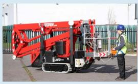
The cable remote control gives the operator a better overview when driving and setting up the lift.
